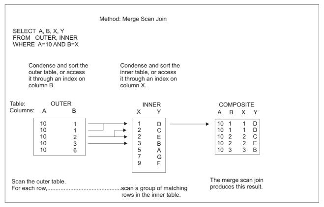
Figure 16. Merge Scan Join
