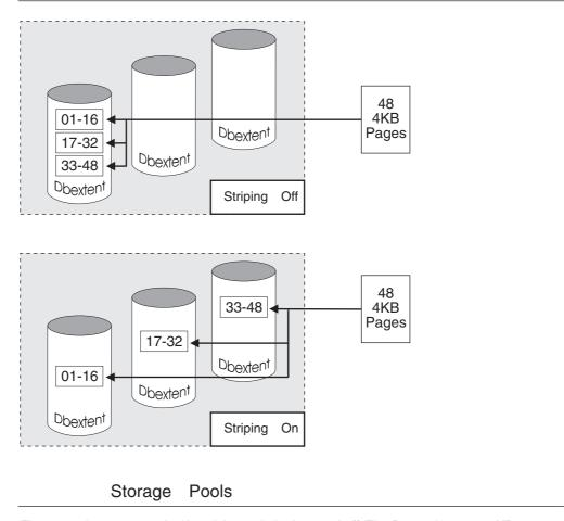
Figure 32. A storage pool with striping switched on and off. The figure shows 48 4KB pages written to DASD with striping on and off.
