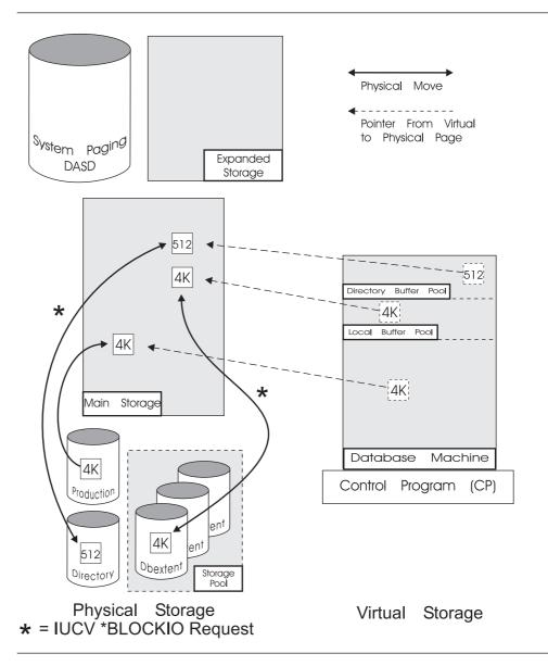
Figure 12. The Standard DB2 Server for VM DASD I/O System. The database manager explicitly directs the operating system to move pages to and from DASD. Once database machine pages are in main storage, they may be moved out to system paging DASD by the paging system. In VSE, pages are moved by VSAM and the database machine is a database partition.
