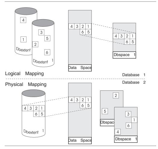
Figure 34. Logical and Physical Mapping
