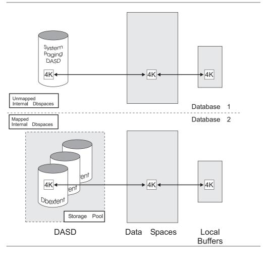
Figure 30. Unmapped and mapped internal dbspaces
