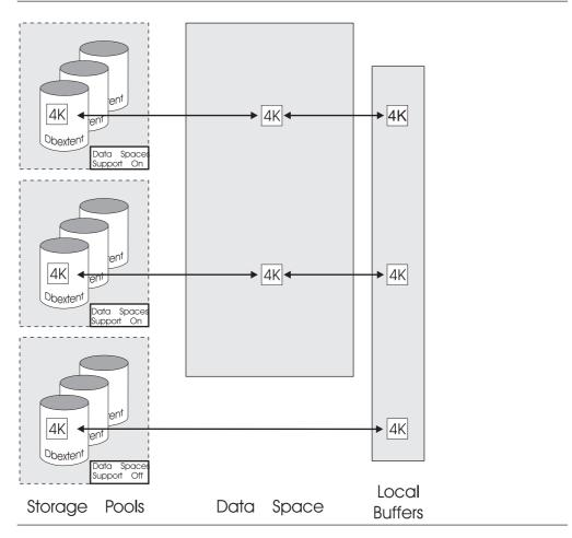
Figure 29. Storage Pools with Data Spaces Support on and off
