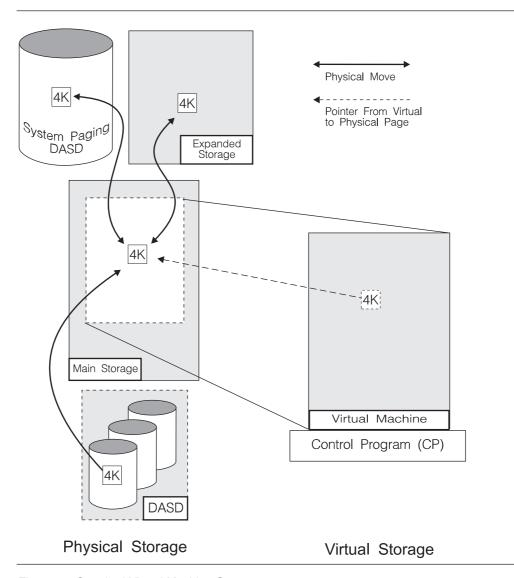
Figure 10. Standard Virtual Machine Storage
