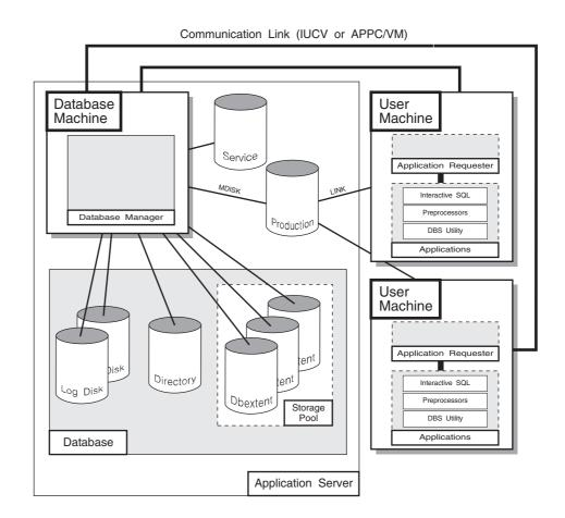
Figure 35. Typical DB2 Server for VM System Setup
