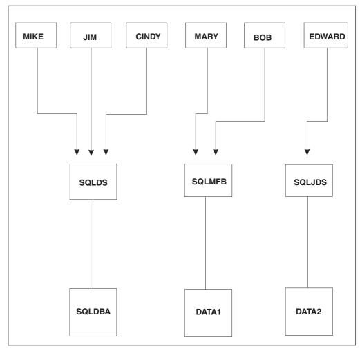
Figure 85. Multiple Users Accessing Multiple Databases
