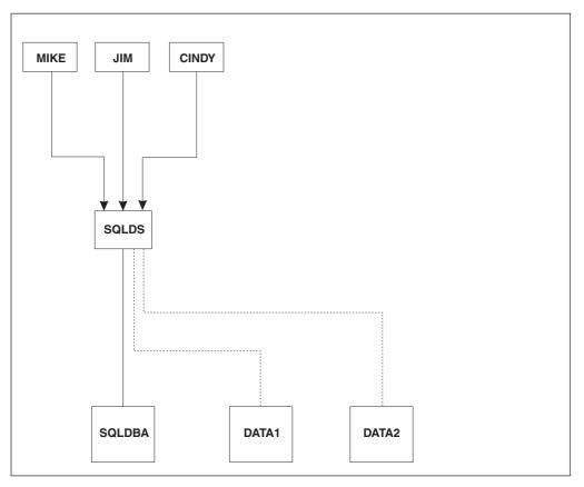
Figure 84. One Database Partition Accessing One Database
