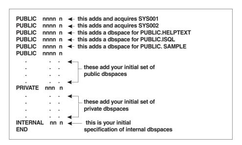
Figure 90. Input Records for Initial Dbspace Definitions
