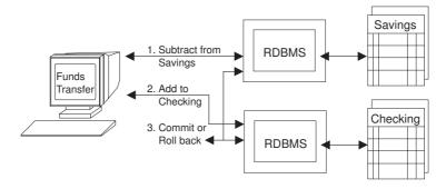
Figure 117. Distributed unit of work
