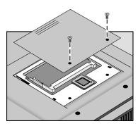
4. Release the two latches at the sides of the RAM board, so the free edge of the board pops up.
