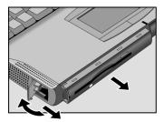
4. Grasp the underside of the module firmly, and pull out.
